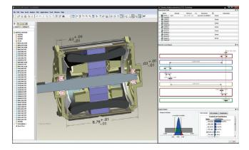
Easy-to-use, powerful tolerance analysis capabilities are now integrated directly into the Pro/ENGINEER design environment with Pro/ENGINEER TAX powered by CETOL Technology.
