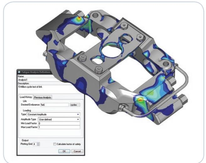
With Pro/ENGINEER Fatigue Advisor, you can easily estimate the number of load cycles your model can sustain before failure.
