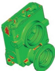
With the confidence of life plot, you can quickly examine the ratio between the calculated life and the target design life.
