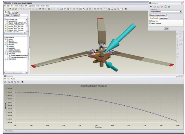
Above: Dynamic forces are applied to the rotor head assembly using Pro/ENGINEER MDO to optimize quality.
