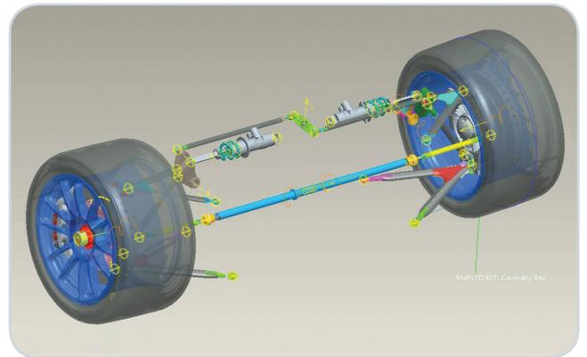
Above: Engineers at Maserati and Dallara use Pro/ENGINEER MDO to simulate real-world forces on this Maserati MC12 race car suspension, reducing the number of physical prototypes and shortening the design cycle.
